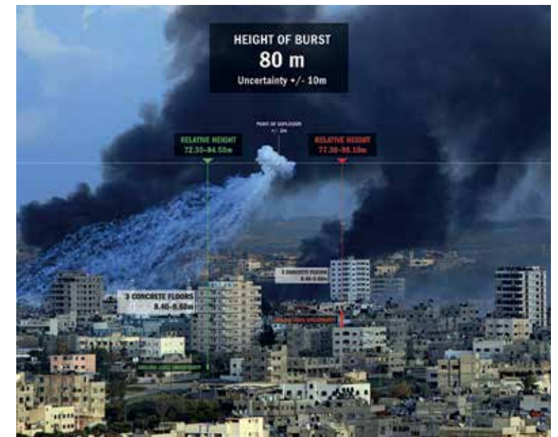
Fig. 2. Photographic analysis. Summary of the methodology used in order to evaluate the height of burst of the M825 WP projectile by using urban structures as reference measures. Rafah, Gaza strip, January 11, 2009. Photo: Iyad El Baba/UNICEF. Visualization: Forensic Architecture and SITU Research.
