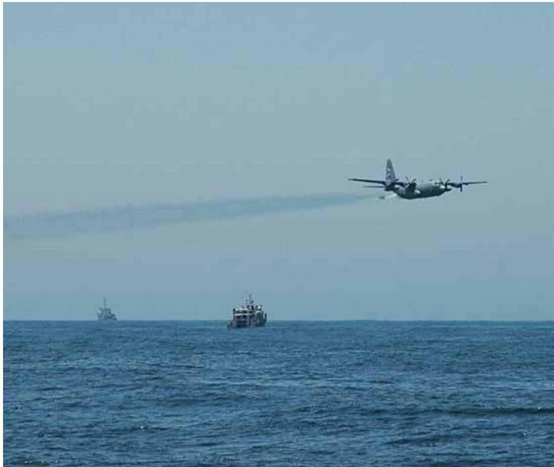
Fig. 2. "Safe Seas": A US Air Force C-130H aircraft sprays water-based dispersant simulators over the Pacific Ocean offshore San Francisco as part of the program Safe Seas Oil Spill Response Exercise, August 9, 2006. Photograph by Capt. Brent Davis. Source: US Air Force.
