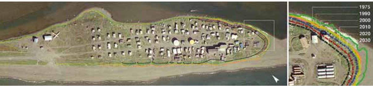
Fig. 4 a, b. The results of the Army Corps coastal erosion study carried out in 2006, marking the former and predicted positions of the shoreline in Kivalina. Source: Army Corps of Engineers Alaska Village Erosion Technical Assistance Program, An Examination of Erosion Issues in the Communities of Bethel, Dillingham, Kaktovik, Kivalina, Newtok, Shishmaref, and Unalakleet , April 2006.
