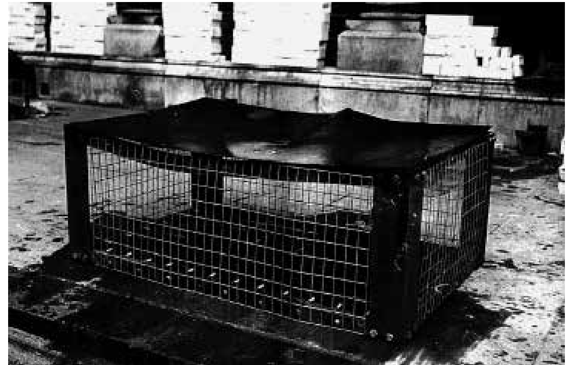
D 2058 Indoor Air Raid Shelter. Tests carried out by the Research and Experimental Department. Flat-topped shelter Type T. This shelter was first tested by dropping a heavy block of concrete weighing 350 lbs from a height of 6 ft above the top. The flat top was only dented. The shelter was then subjected to a second test in which a floor weighing 1,800 lbs and pivoted at one side was dropped 6 ft 6 inches and with a swinging action so that it struck one top edge of the shelter as it fell, simulating the manner in which the floor of house usually collapses. The steel angle at the top edge was bent.
