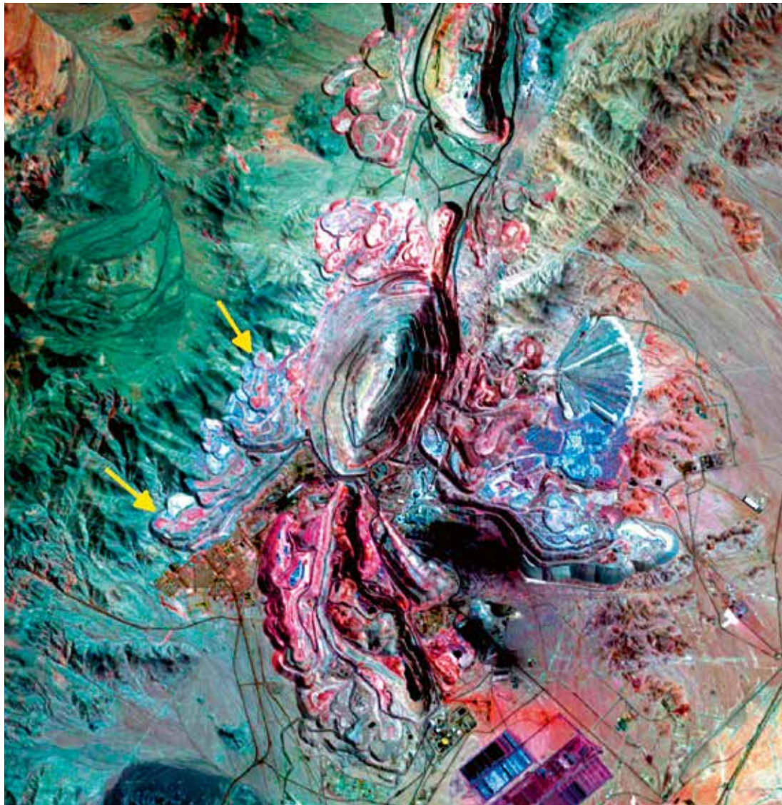
Fig. 1. Chuquicamata copper mine. Color composite image enhancing the presence of jarosite, a result of oxidized pyrite, typically found in copper mining rock waste. Landsat 8 OLI, April 2013. Source: US Geological Survey. Composite image: Godofredo Pereira.
